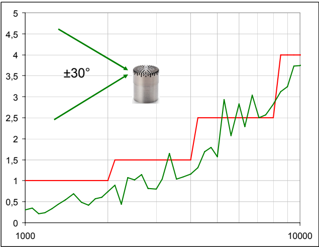
Fig. 4: In green directional response of a 1/2' microphone for \theta = 30^\circ (reference direction 90^\circ ); in red, tolerance values of IEC 61672-1 without expanded uncertainty
