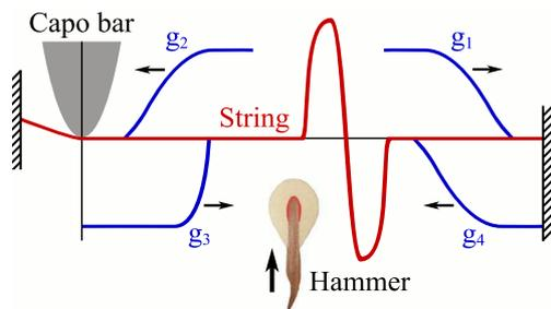
Figure 2: Scheme of capo bar-string interaction. Functions  $g$  are the traveling waves.
