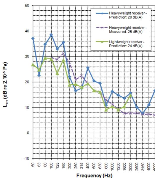
Figure 11: Predicted structure-borne noise - 2 1/s
