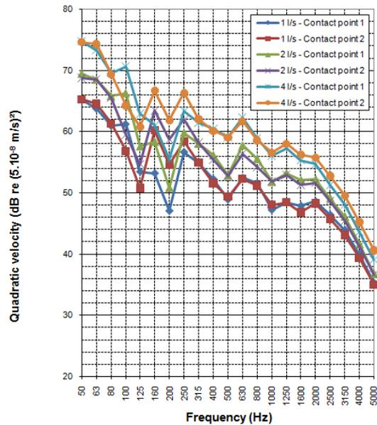
Figure 6: Measured source free velocities
