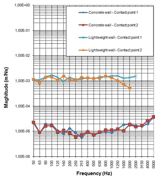
Figure 7: Measured receivers point mobilities
