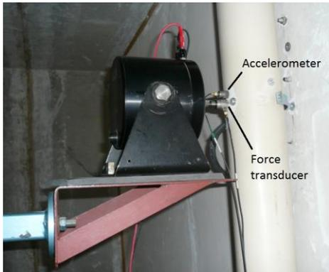
Figure 4: Experimental setup used for source point mobility measurements
