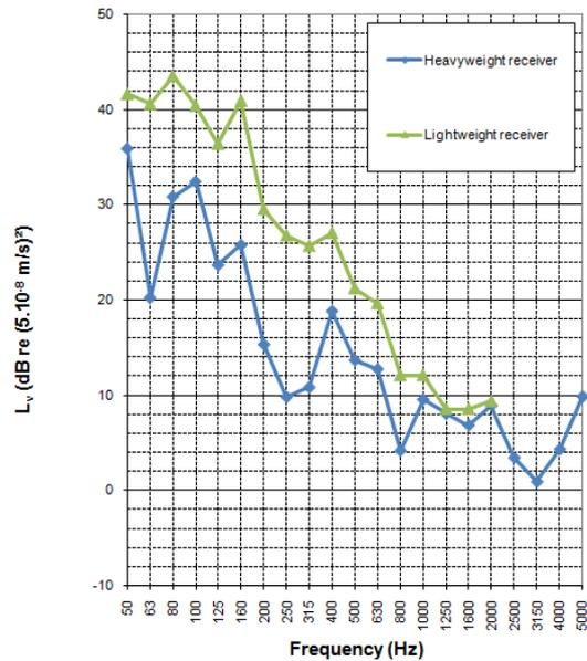
Figure 9: Predicted velocity level - 2 l/s
