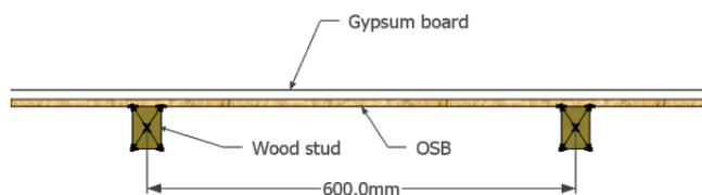
Figure 3: Lightweight separating wall under study (top view)
