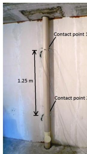
Figure 2: View of the waste water pipe installed on a heavyweight separating wall
