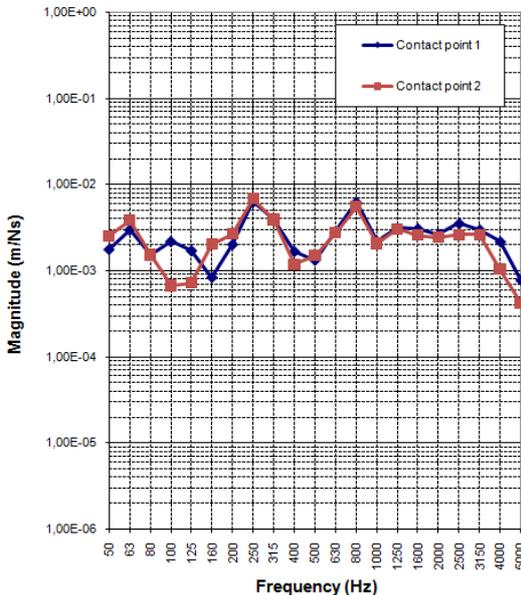
Figure 5: Measured source point mobilities
