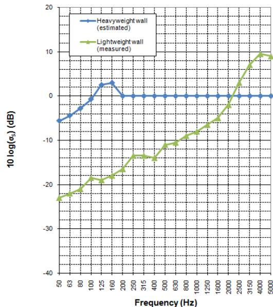
Figure 10: Radiation efficiency values considered
