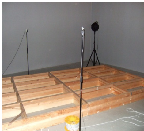
Figure 3. Measurements of sound absorption coefficient in reverberant chamber according to Standard UNE-EN ISO 354:2004
