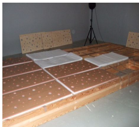
Figure 4. Measurements of sound absorption coefficient in reverberant chamber according to Standard UNE-EN ISO 354:2004
