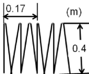
Fig. 5 M shaped wedge test specimen for anechoic measurement.
