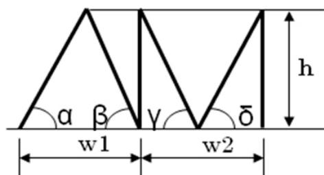
Fig. 1 Geometric parameters of M shaped noise barrier.
