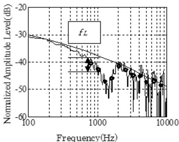
Fig. 2 Measurement example of the cut-off frequency  $f_L$
