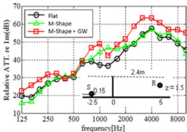
Fig. 7 Measurement example of the relative attenuation (re. 1 m in free field) of flat edge barrier and M shaped barrier with / without glass wool board behind. The shape parameter of the latter is  $h = 340$  mm,  $w_1 = w_2 = 360$  mm, and  $\alpha = \beta = \gamma = \delta = 62^\circ$ .
