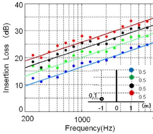
Fig. 4.1 Comparison of the insertion loss of the flat top edge between measurement (circle) and calculation (solid line).
