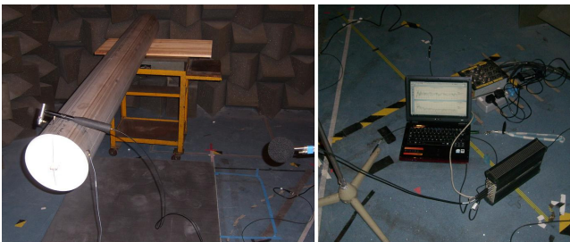
Figure 6: Experiment set up to explore air column and structural responses of tubes required for Aeolus.
