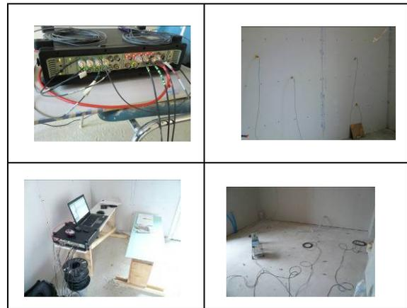
Figure 4: Vibration level difference in situ measurements
