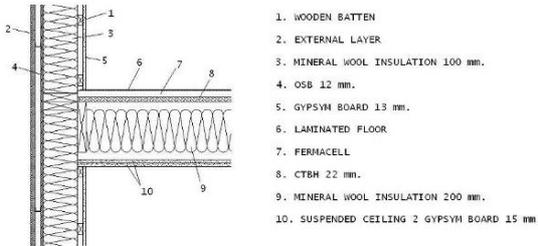
Figure 3: Elements composing the Floor and Façade Junction
