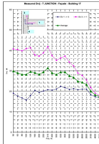
Figure 5: Measured T junction Floor-Façade. Paths 1-3.
