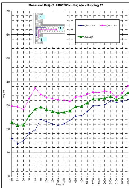
Figure 7: Measured T junction Floor-Façade. Paths 1-4.
