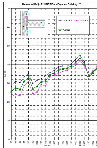
Figure 6: Measured T junction Floor-Façade. Paths 3-4
