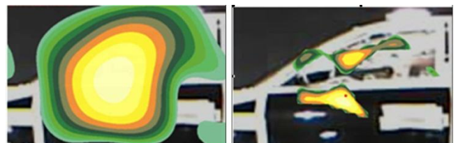
Fig. 5: Sound Intensity maps based on beamforming measurements in a wind tunnel. Left: delay and sum method. Right: Refined beamforming method.
