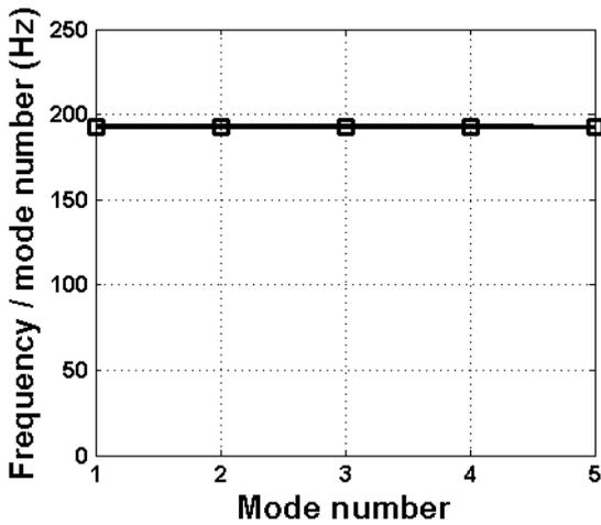
Figure 5: The frequency divided by the mode number of the fundamental wave and the harmonics
