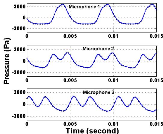
Figure 2: AC-coupled pressure waves in the time domain at different temperature differences across the stack at three different axial locations along the resonator
