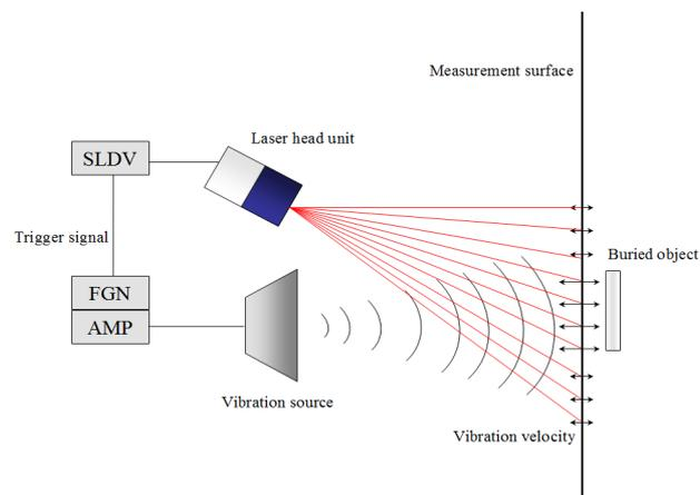
Fig.1: Fundamental concept of NCAI.
