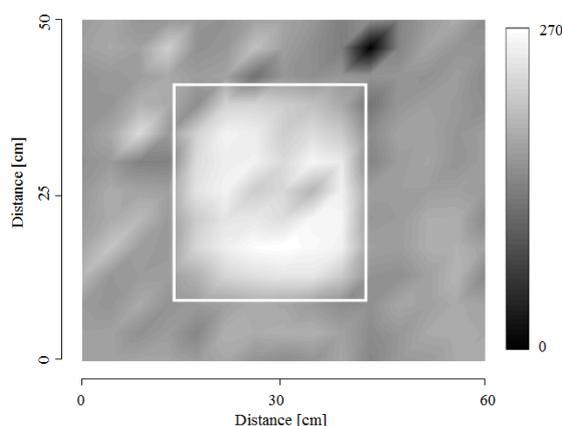
**Fig. 10:** An applying example of the optimum frequency range method (OFR method). In this case, frequency range from 1300 to 1600 Hz are integrated .
