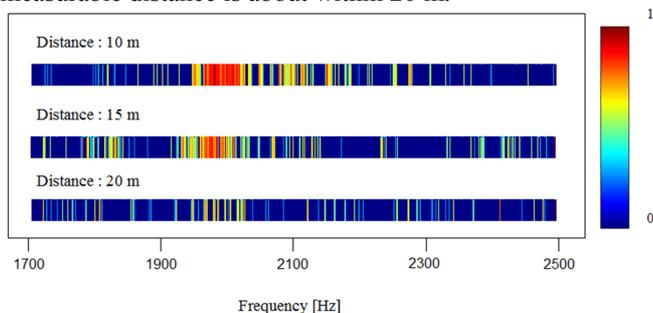
**Fig. 8:** Brightness image of the frequency response of the vibration velocity. The distance between a concrete test piece and a LRAD is 10, 15 and 20 m.
