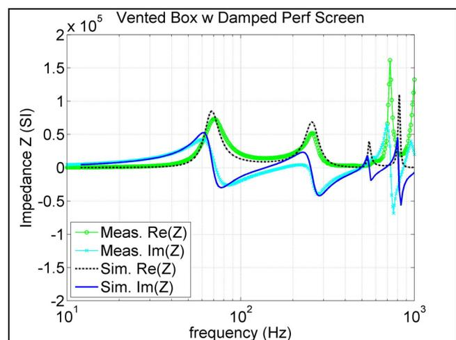
Fig.14 Vented box with damped perforated wall design,
