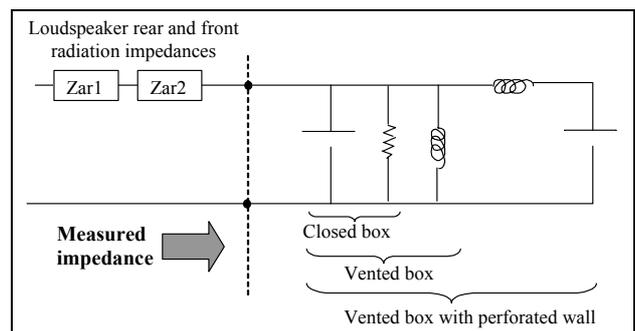
Fig.4 Current electroacoustic modelisation of enclosures
