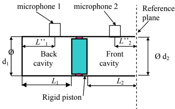
Fig.1 Schematic drawing of the impedance measurement sensor and notations
