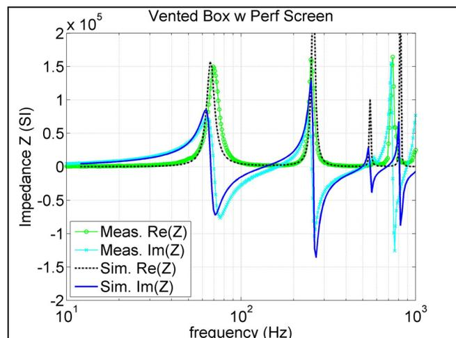
Fig.13 Vented box impedance with perforated wall design
