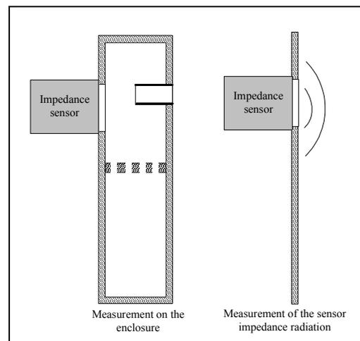
Fig.7 Set up for the measurement of  $Z_{radiation}$
