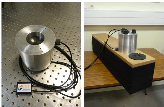
Fig.2 View of the impedance sensor and its application to loudspeaker enclosure design
