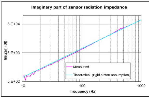
Fig.8 Imaginary part of the sensor radiation impedance
