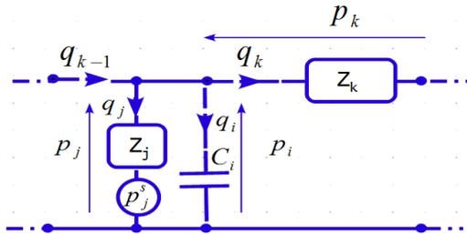
Fig.5 : equivalent circuit of an elementary cell of the discrete simulation scheme of fig. 6 (impedance analogy)
