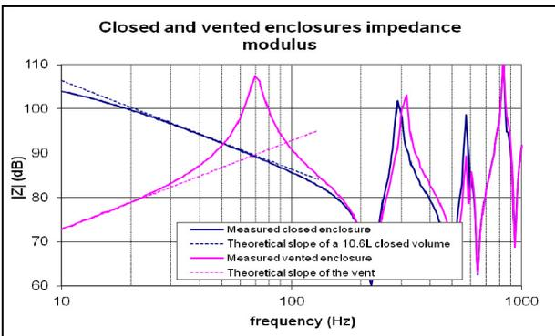
Fig.9 Acoustic impedances of closed and vented enclosures
