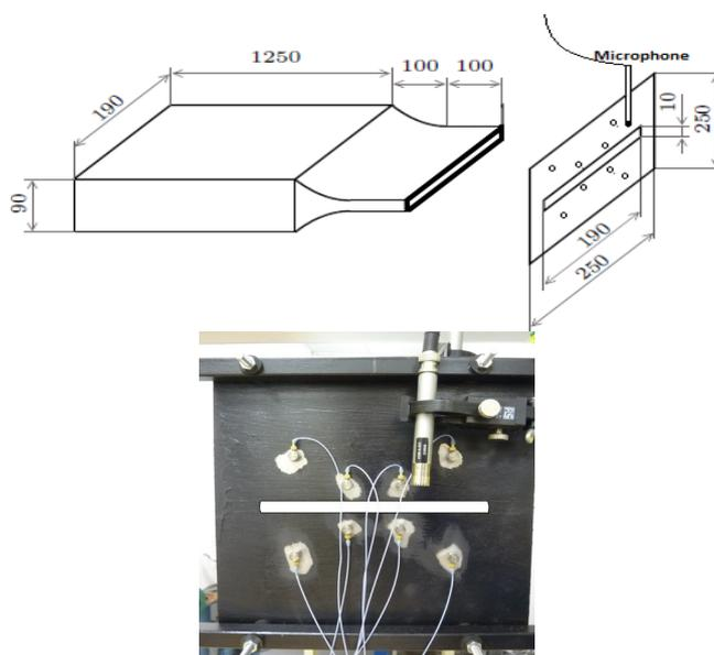
Figure 1: Experimental apparatus
