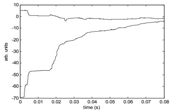
Figure 5: Intensity Schroeder plot along directions X (bottom line) and Y (top line).
