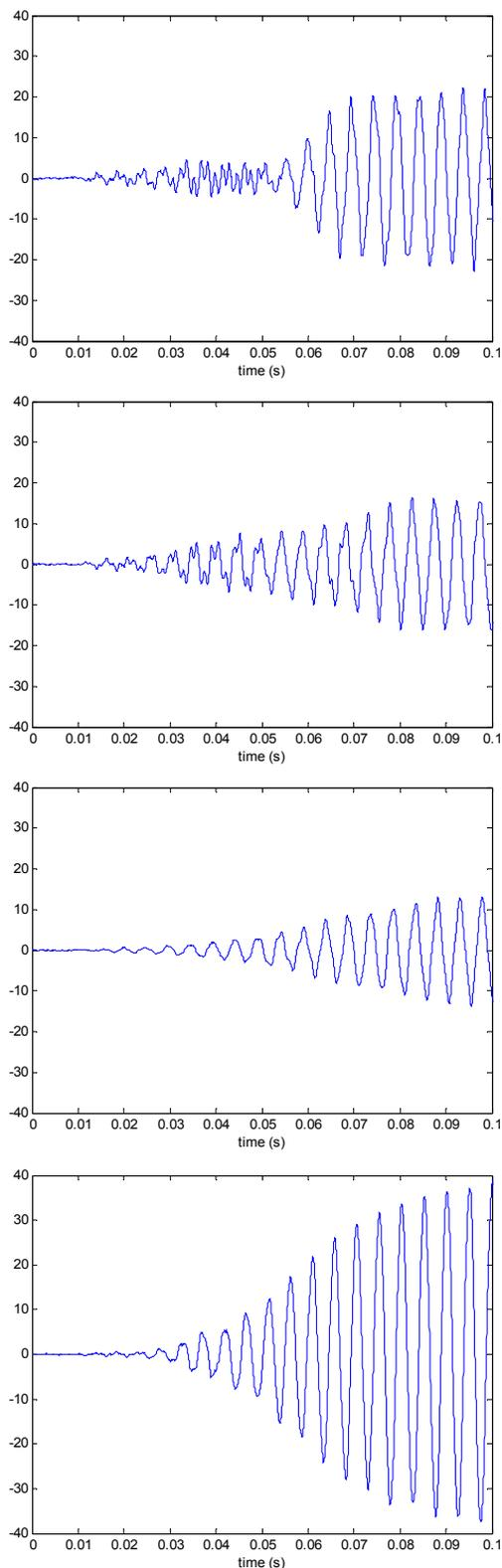
Figure 7: From top to bottom, pressure and X,Y,Z components of acoustic velocity of an organ pipe tone synthesized by convolution with quadrasonic impulse response of Fig. 3.
