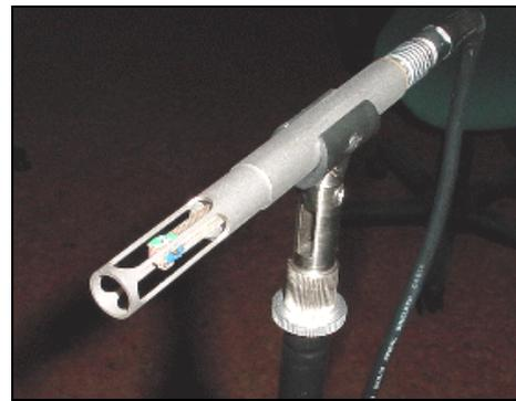
Figure 1: The 3D Microflown probe on the tripod.
