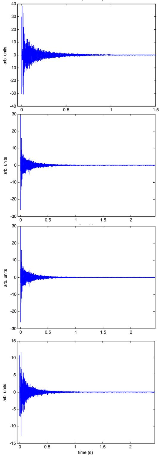
Figure 3: From top to bottom, pressure and X,Y,Z components of acoustic velocity impulse responses of the conference room.
