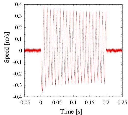
Fig. 18. Continuous reciprocation motion at 100Hz with energy circulation drive.
