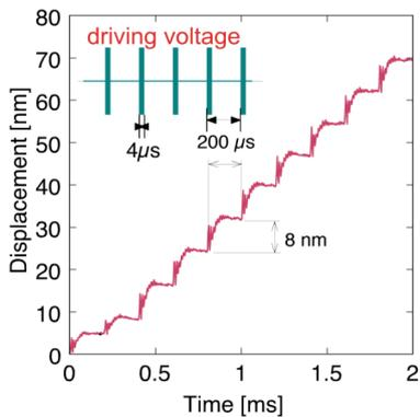
Fig. 13. Stepping motion with 40 waves burst drive.
