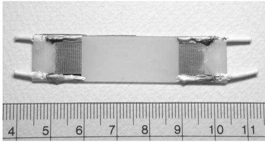
Fig. 3. Surface acoustic wave device for stator transducer; 128 y-rot. x-prop. LiNbO<sub>3</sub> and 9.6 MHz driving frequency.
