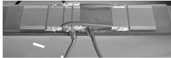
Fig. 16. Stator transducer for energy circulation drive.
