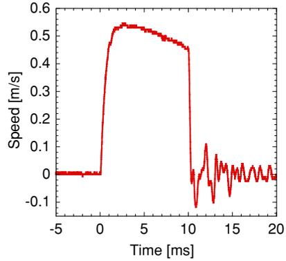
Fig. 7. Transient response; driving voltage and pre-load were 125 V and 113 N
