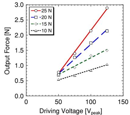
Fig. 10. Output force vs. driving voltage.
