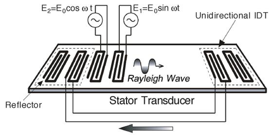
Fig. 15. Driving method of energy circulation for efficiency improvement.
