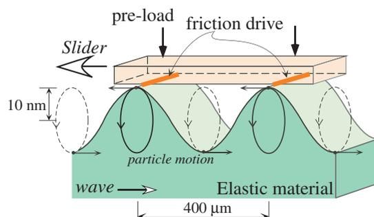
Fig. 2. Principle of surface acoustic wave motor using Rayleigh wave.
