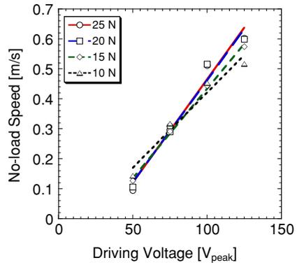
Fig. 9. No-load speed vs. driving voltage with a function of pre--load.
