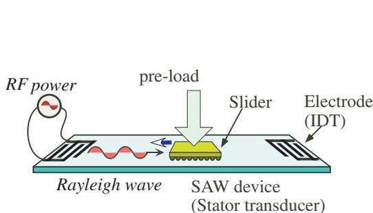
Fig. 1. Schema of surface acoustic wave motor.
