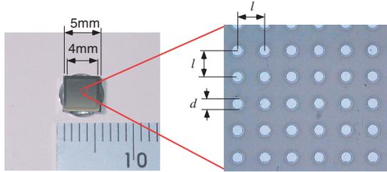
Fig. 5. Silicon slider and its surface view with SEM.
