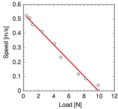
Fig. 8. Speed versus mechanical load characteristics estimated from Fig. 7.
