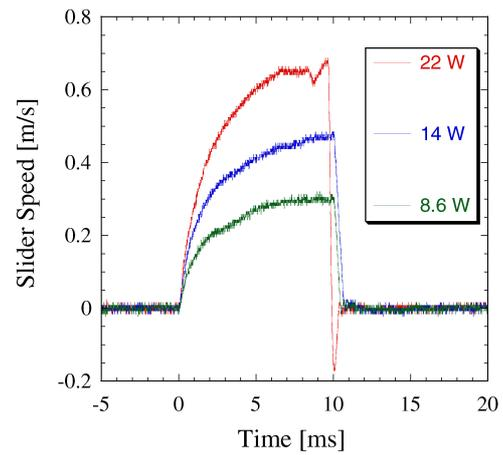
Fig. 17. Transient response of the energy circulated driving motor.
