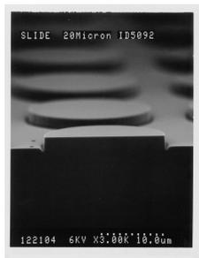
Fig. 6. Silicon slider surface cross view with SEM.
