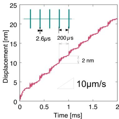
Fig. 14. Stepping motion with 25 waves burst drive.
