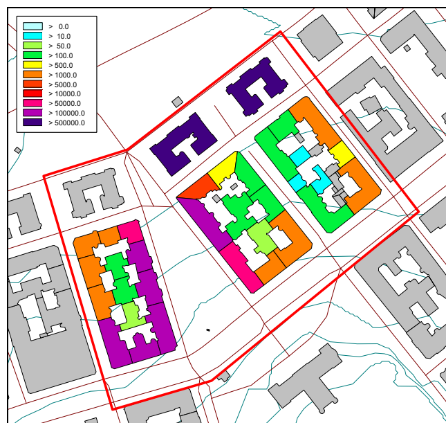
Fig.9 The figure shows the results from a NERS-analysis including the quiet side. The noise score on the quiet sides have been calculated using the shifted noise score function. The effect is most clear at the buildings inside the courtyards.
