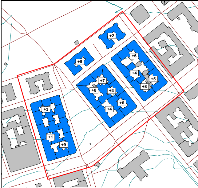
Fig.5 The figure displays the difference between measured values delivered by the city of Gothenburg and the levels calculated with the Nordic prediction model. All sound levels in dB(A).
