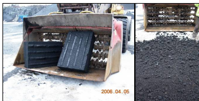
Fig. 1. To the left: bitumen wetted rubber blocks in the ALLU. To the right: rubber/bitumen mix as powder after dissolving the block in the ALLU.
