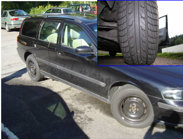
Fig. 3 Test vehicle Volvo V70 Bi-fuel used for both Pass-by and CPX-tests. The reference test tyre was of type Goodyear Hydragrip 195/65R15.
