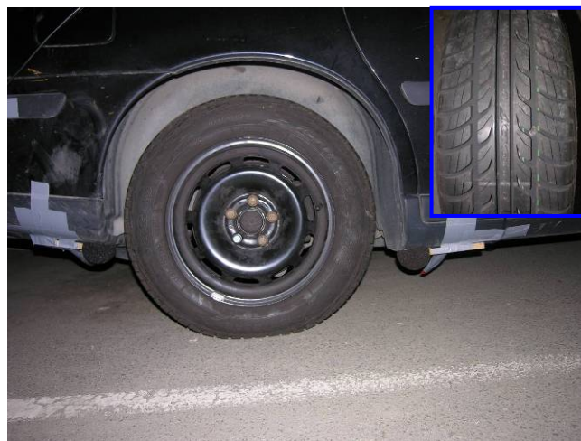
Fig. 7 Test vehicle Volvo V70 Bi-fuel used for both the Pass-by and CPX-tests. The test vehicle was supplied with test tyres of type Goodyear Hydragrip of type 195/65R15.
