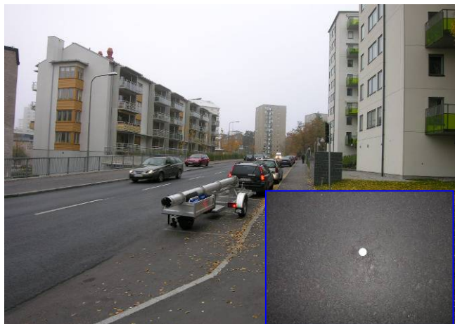
Fig. 4 Reference road surface of type AC 16 at Kirunagatan in Stockholm. A Swedish 5 krona coin has been used in the close-up for reference. The picture also shows the single wheel trailer for tyre/road measurements used in this study.
