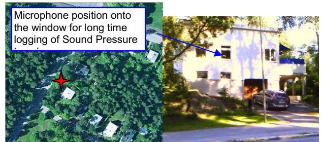
Fig. 9 Microphone position during traffic noise logging.
