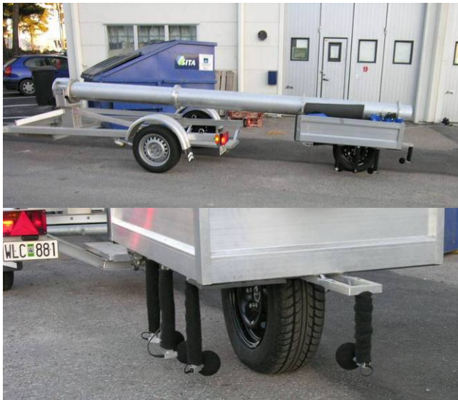
Fig. 8 Photo of the single wheel trailer for measurements of tyre/road noise here mounted with the reference test tyre Goodyear Hydragrip 195/65R15.
