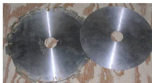
Figure 5: Diamond-infused cutting blade and non-cutting spacer
