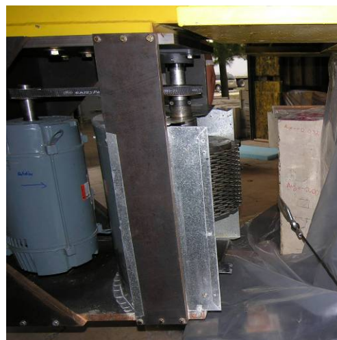
Figure 4: Grinding apparatus with stack of diamond cutting blades
