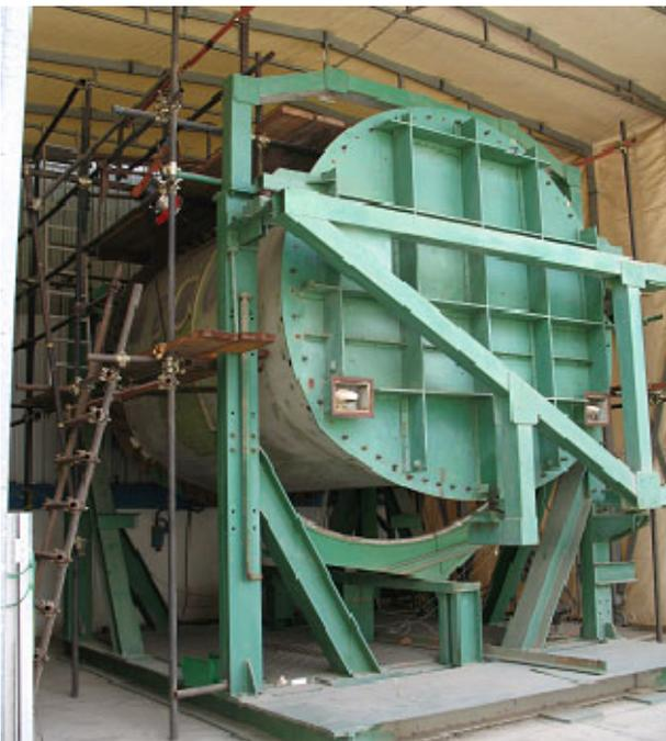
Fig.1 Mock-up of the ATR 42 aircraft and constraining structure.
