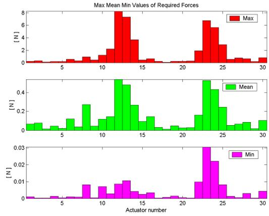
Fig.7 Required control force values for the control actuators in their optimal configuration
