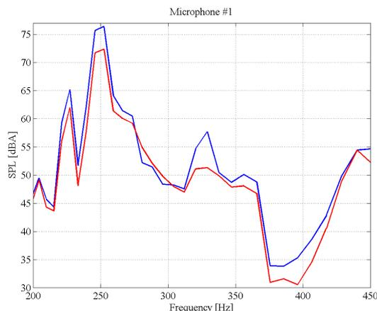
Fig.14 Primary field from specs: control off (blue), control on (red)
