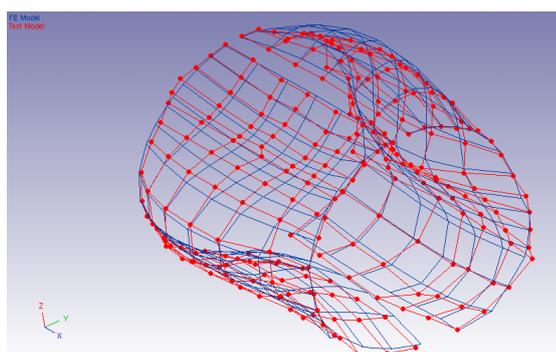
Fig.4 Mode shape pair comparison - FEA 67.6Hz - EMA 61.94Hz - MAC 76%
