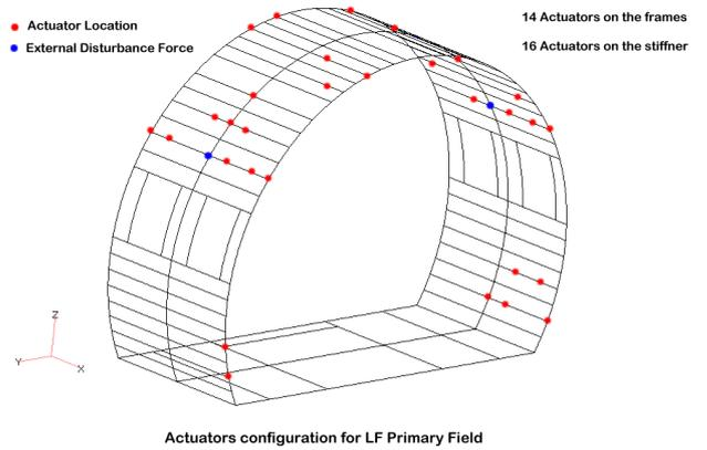
Fig.8 Optimal actuators placement configuration – low frequency disturb force field
