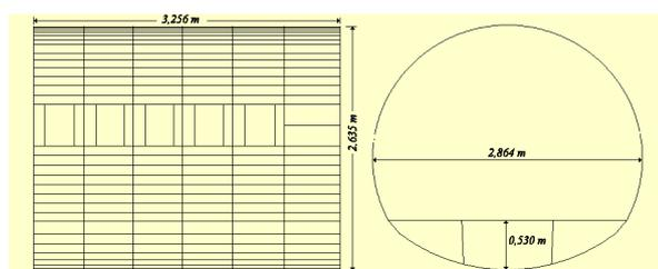
Fig.2 Overall dimension of the fuselage mock-up
