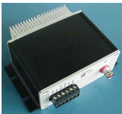
Fig.10 Light hybrid amplifier: Supply voltage 16...30 V, Input voltage range: 0...4 V, Output current range: 0...4 A, Operating frequency range: 0...15 kHz,  $-3^\circ$  phase shift at 1.1 kHz
