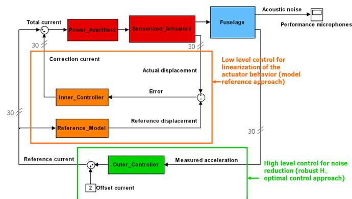
Fig.11 Overall noise and vibration control scheme (30 control channels)
