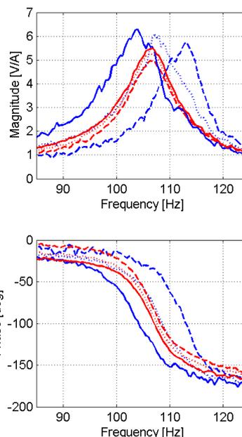
Fig.12 : Actuator behaviour at different current: control off (blue), control on (red)
