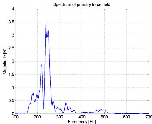
Fig.13 Primary force field from specifications
