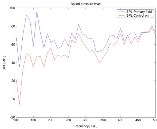
Fig.6 Mean interior noise reduction for the optimal actuators configuration
