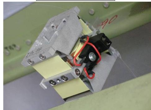
Fig.9 Actuator (with integrated optical sensor) schematic and actual installation on a fuselage stringer
