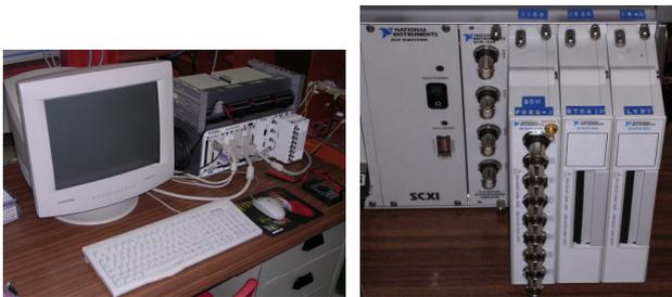
Fig. 15: Acquisition system and detail of input cards.
