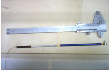
Fig 7: The micro-hammer.
