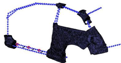
Fig. 6 Hybrid TM-FEM model of a real automotive hollow body network.
