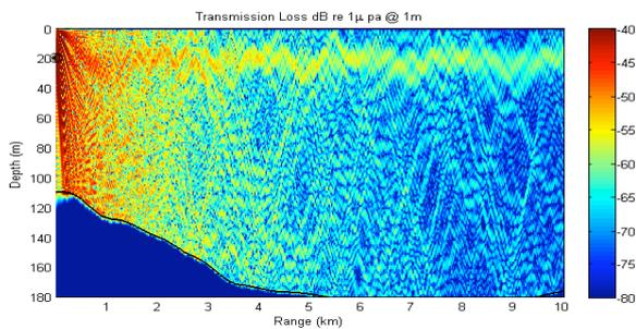
Figure 3: Acoustic TL modeling (900 Hz)
