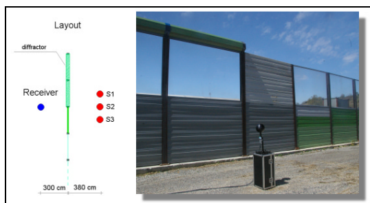
Fig. 15 Measurement on noise barrier
