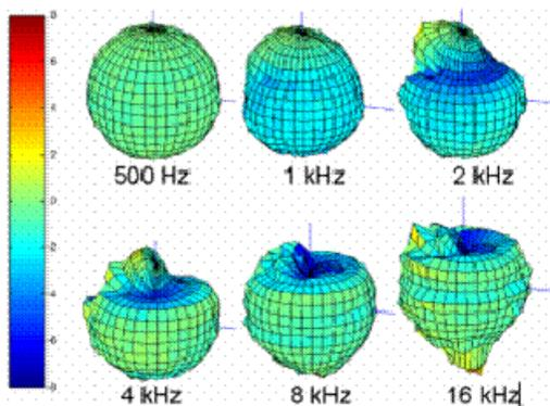
**Figure 16** 3D plot of the effect of a cap on directivity pattern of the artificial head
