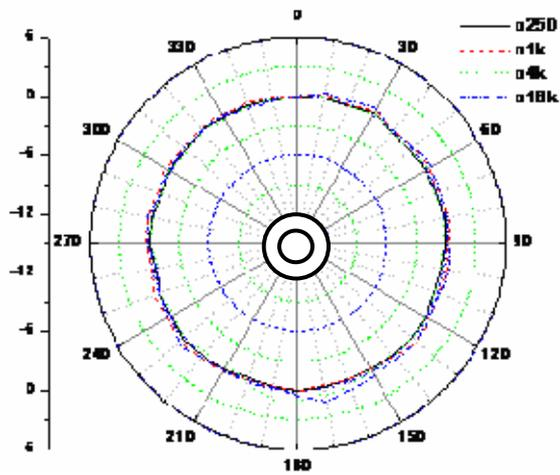
Figure 9 2D polar plot of a straw hat effect on directivity pattern of the artificial head in horizontal plane
