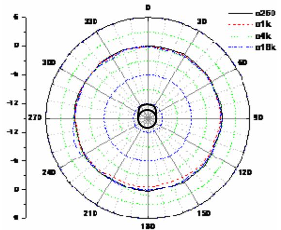
Figure 11 2D polar plot of a cap effect on directivity pattern of the artificial head in horizontal plane
