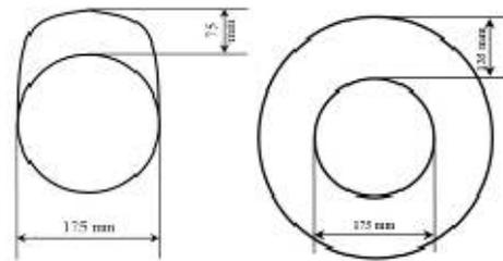
**Figure 4** Sporting cap (left) and straw hat (right) dimensions and shape (top projection)
