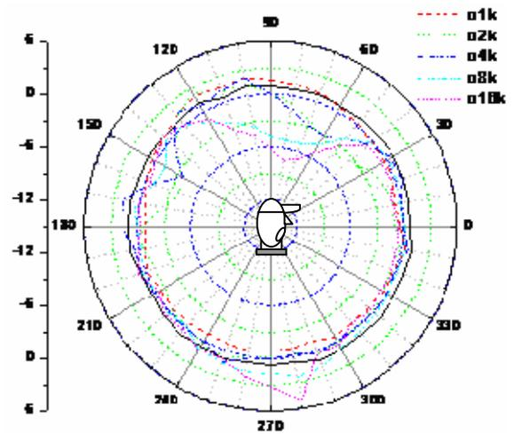
Figure 12 2D polar plot of a cap effect on directivity pattern of the artificial head in vertical plane
