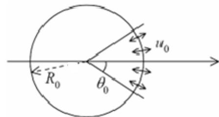
**Figure 1** Mathematical approximation of a human speaker head with radially vibrating spherical cap set in a sphere
