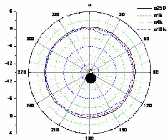
**Figure 7** 2D polar plot of a wig effect on directivity pattern of the artificial head in horizontal plane
