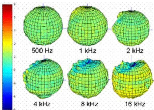
**Figure 15** 3D plot of the effect of a straw hat on directivity pattern of the artificial head
