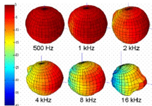
Figure 13 3D plot of detailed directivity pattern of the artificial head
