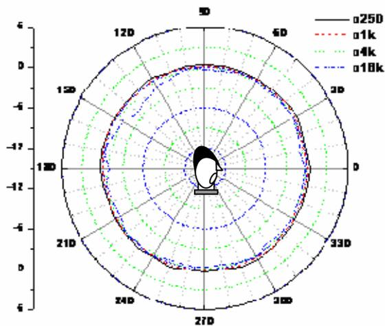
Figure 8 2D polar plot of a wig effect on directivity pattern of the artificial head in vertical plane
