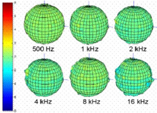
**Figure 14** 3D plot of the effect of a wig on directivity pattern of the artificial head
