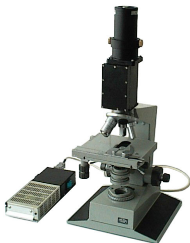
Fig.2. Double-AOTF microscopic monochromator with CCD camera.
