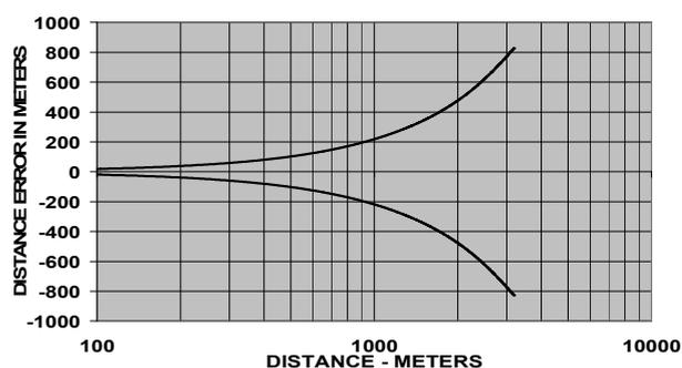
Figure 3: The 95% C.I. from Figure 2, as derived from Table 2 uncertainties, for the example case, presented in terms of the error of estimating the distance to a given sound level isopleth.
