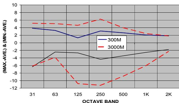
Figure 6: Range of results for a recent ASTM Round Robin far field propagation modeling test. The test case was a point source and a receiver, each at 1.5 meters above a flat, grassy ground plane with the receiver located at either 300 or 3,000 meters from the source. An infinitely long perpendicular 3-meter high barrier wall was located 10 meters from the source. Ambient conditions were assumed to be calm (for some models
