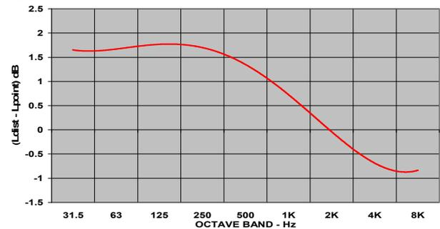
Figure 7 – Distributed vs. Point Source Evaluation: Differences in octave band sound pressure level, plotted as the difference between the level for the distributed source model (each of 14 components modeled as 54 points) minus the level with each of the 14 components modeled as an individual point, at a far field position 1.5 meters above grade and 240 meters from the source, with a 10 meter high barrier located 33 meters from the source.
