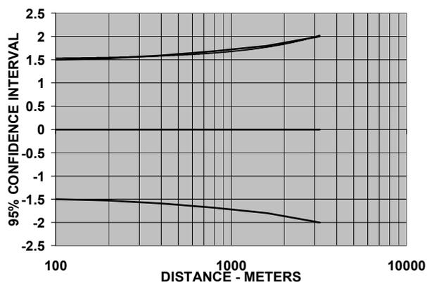
Figure 1: Applying the 95% C.I. uncertainties of Table 2 to an example case of a simple cycle 100MW class gas turbine far field A-weighted sound levels.
