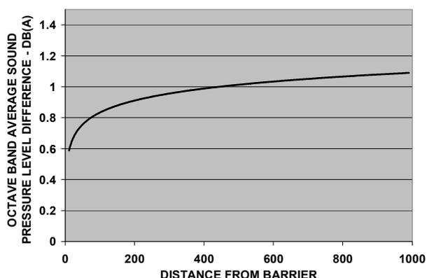
Figure 9 – Distributed vs. Point Source Evaluation: The trend of the differences in the average of the nine standard octave bands, plotted as the difference between the average for the case of the distributed source model (each of 14 components modeled as 54 points) minus the average for the case of each of the 14 components modeled as an individual point, as a function of the distance from the source, in meters, with a 10 meter high barrier located 33 meters from the source.
