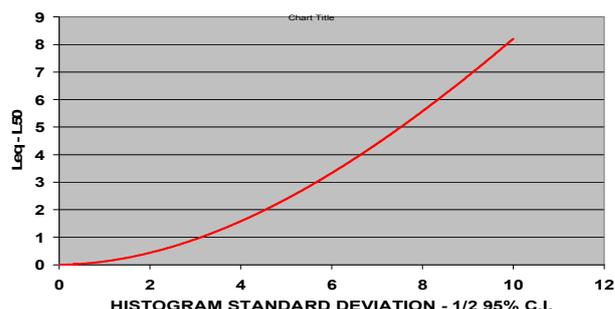
Figure 4: Atmospheric Diffusion Effect: Difference between the mean,  $L_{50}$ , and the equivalent,  $L_{eq}$ , sound level of any given normal distribution histogram as a function of the standard deviation of the histogram.
