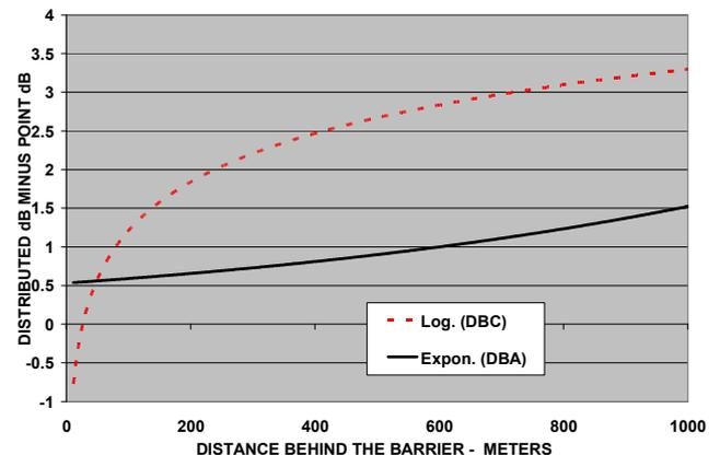
Figure 8 – Distributed vs. Point Source Evaluation: Differences in A-weighted (bottom curve) and C-weighted (top curve) sound level, plotted as the difference between the level for the distributed source model (each of 14 components modeled as 54 points) minus the level with each of the 14 components modeled as an individual point, at far field positions 1.5
