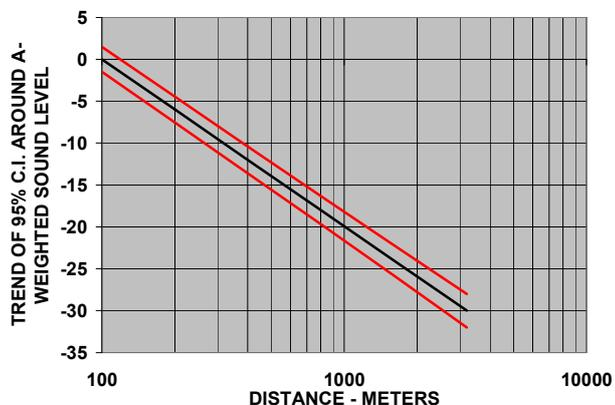
Figure 2: Radial Trend of the example simple cycle gas turbine far field A-weighted sound levels with the 95% C.I. of Figure 1 based upon the Table 2 uncertainties.
