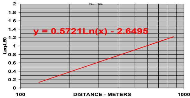
Figure 5: Atmospheric Diffusion Effect: Log-Trend line of an actual case history showing the result of a progressive broadening of a histogram with increasing distance from the source. The trend line is for the difference, in decibels, between measured  $L_{eq}$  and measured  $L_{50}$  for the 25 Hz one-third octave band from a pair of simple cycle gas turbines. The distance is from the approximate acoustical center of the turbines.
