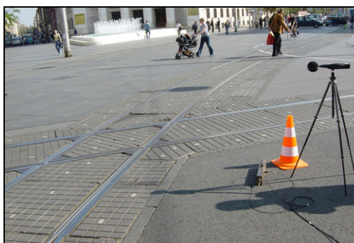
Fig.7 Sound level meter and accelerometers (MP-2).
