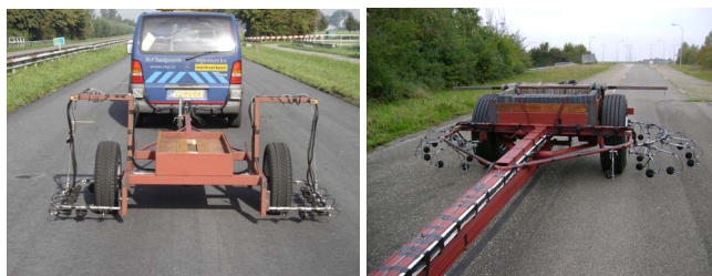
Fig. 7 Near-field rolling noise trailers for passenger car tyres (left) and truck tyres (right)
