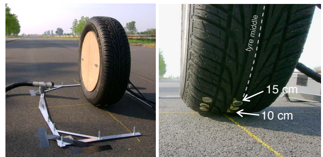
Fig. 1 Near-field point source array (left), mock-up with two microphones mounted in the tyre tread (right)
