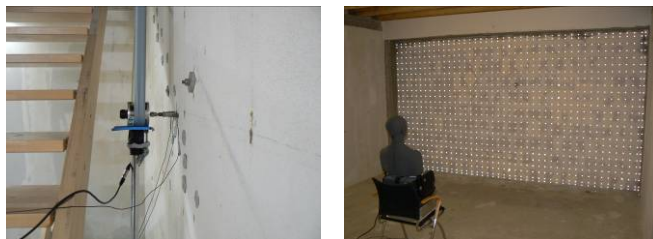
Fig.10 Shaker attached to the wall (left) and laser scanning grid with 1100 points (right)
