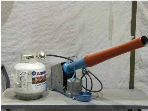
Figure 6: Photograph of the liquid propane cannon source
