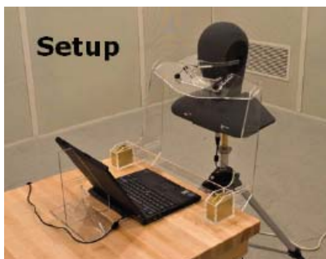
Fig.1 Binaural recording setup with alignment fixture.
