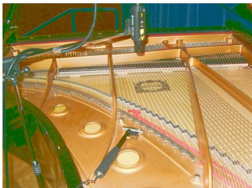
Figure 2: Photo showing the C7 piano with the B&K impact-hammer and the Polytech laser-head utilized during the measuring sessions.
