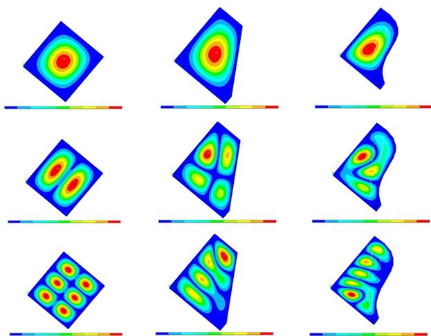
Figure 5: Modes 1st, 5th and 8th of three types of plates. Left, rectangular orthotropic. Center, trapezoid shaped orthotropic. Right, piano shaped orthotropic with ribs and bridges. Plots are not equally scaled. All of them show motionless edges, which corresponds to boundary conditions.
