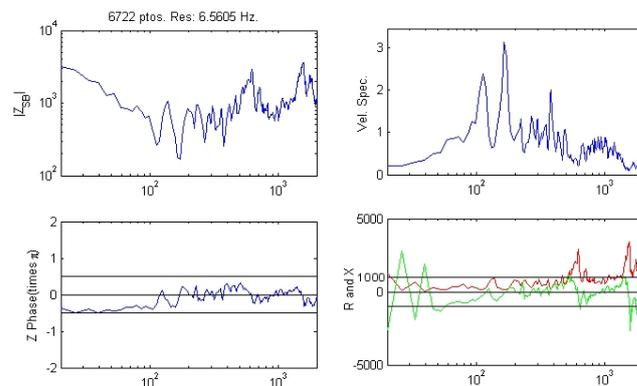
Figure 3: Measurement results when exciting the point of 24-th note in the bass bridge. The modulus and phase of  $Z_{SB}$  are shown in the left side. The upper-right plot shows the velocity spectrum and its peaks indicate the modes frequencies. The lower-right plot shows both the real (always positive valued) and imaginary parts of the measured impedance.
