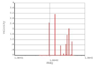
Figure 6: Velocity simulated at about 24-th note point, considering an undamped piano plate. The distribution of levels is similar to the measured ones.
