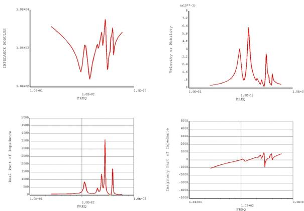
Figure 7: The complete simulation results. A perfect resemblance of the measures is impossible, but the similarity is good enough. Impedance measures includes the effect of the strings impedances, which produce 'small irregularities' in the measured curves.
