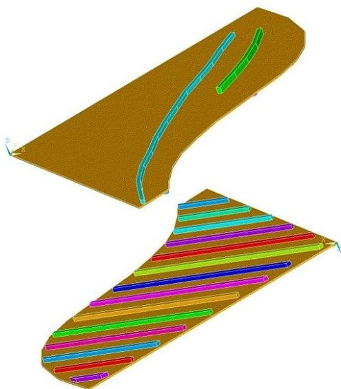
Figure 4: The designed model of the soundboard with ribs and bridges used in FEM calculations. The shapes of soundboard and bridges follow the Steinway's patent.
