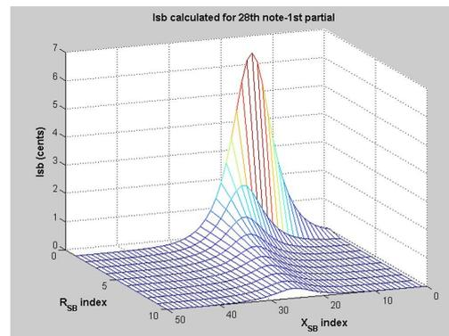
Figure 1:  $I_{SB}$  deviation calculated by Ortiz et al.[5] for the first partial of 28-th note as a function of a range of  $R_{SB}$  and  $X_{SB}$  values, represented by indexes.  $R_{SB}$  indexes correspond to a range linearly spaced from 100 to 1900 kg/s.  $X_{SB}$  indexes correspond to a range logarithmically spaced from 0 to  $10^{+6.5}$  kg/s.
