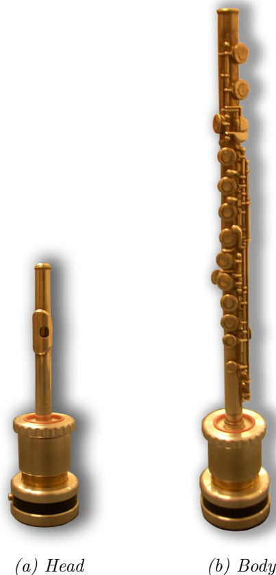
Figure 1: BIAS Head with flute parts. The player can simulate the embouchure during the measurement of the head.
