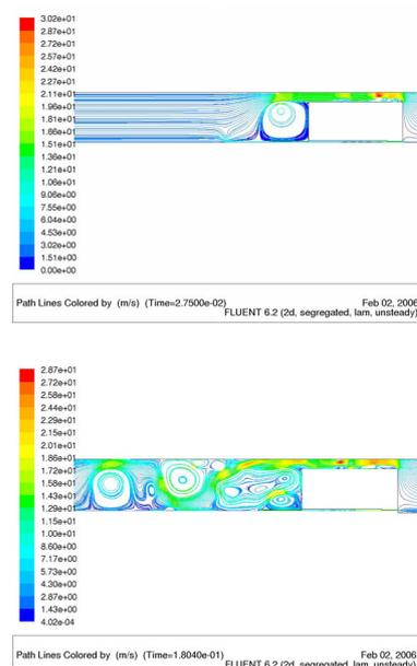
Figure 4- Pathline of flow field about standard elevator cab. Two dimensional model.  $Re=3.5 \times 10^5$
