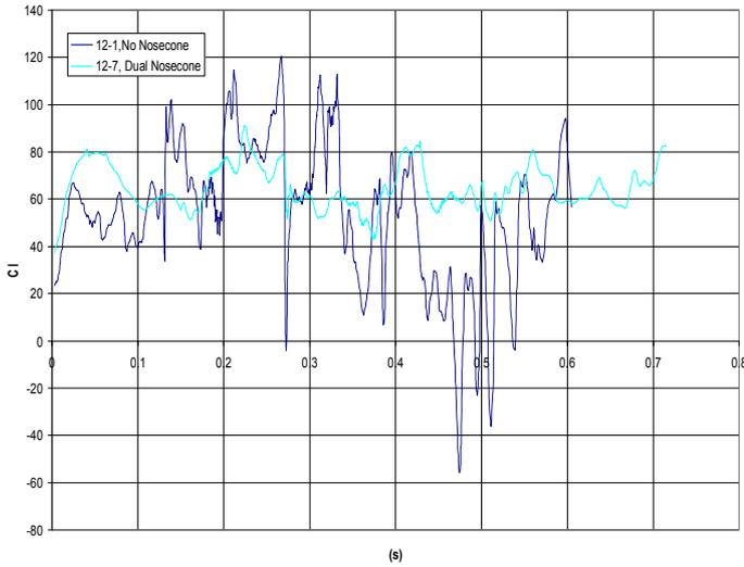
Figure 5-Comparison of Side force due to vortex shedding around the elevator cab
