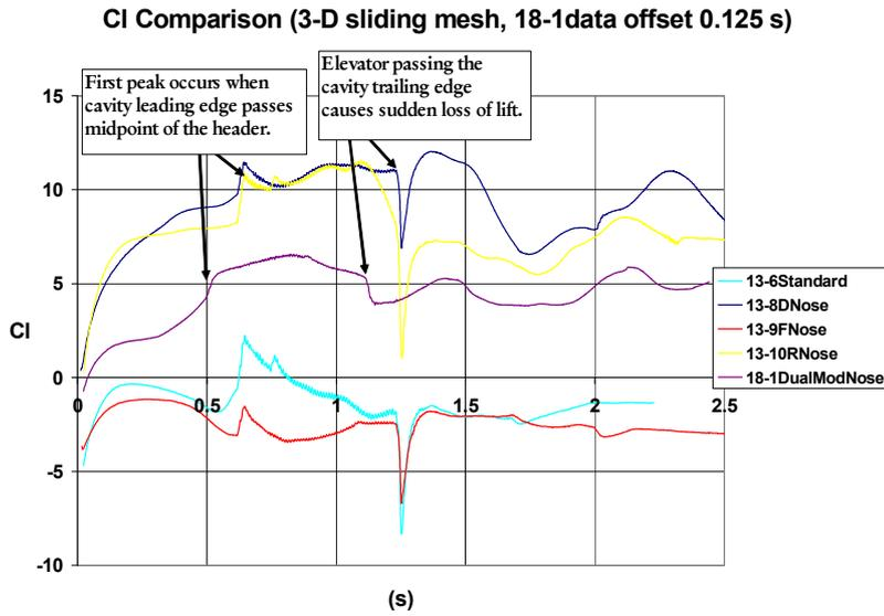
Figure 10- Comparison of side forces of a 3D elevator cab model with different types of nose cones
