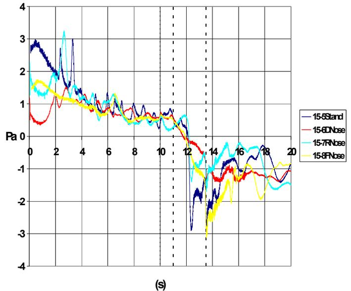
Figure 7- Comparison of cavity pressure due to the flow produced by a standard elevator and with nose cones
