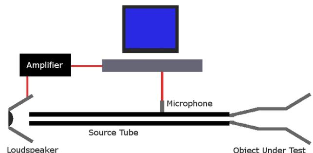
Fig.1 Acoustic Pulse Reflectometry Apparatus.
