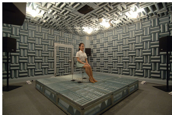
Fig.2 Reproduction system set in a semi-anechoic room.
