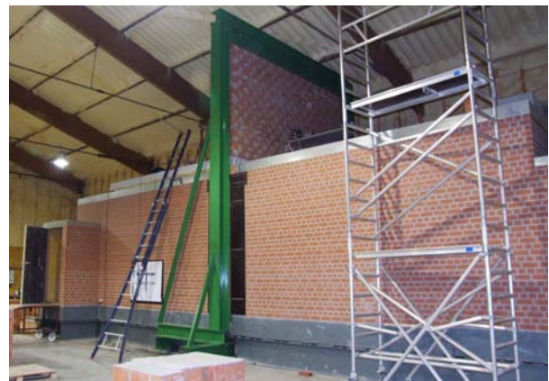
Fig. 5.a System of steel beams to load the walls
