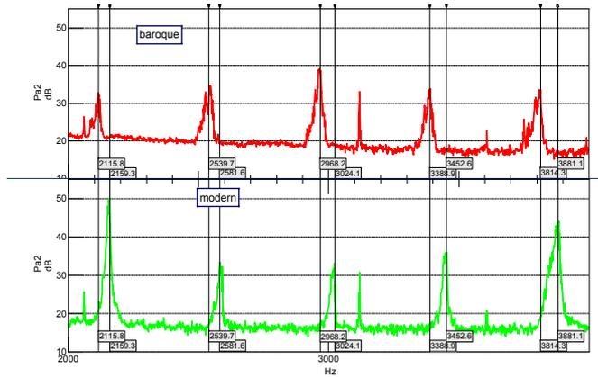
Fig 3: Sound pressure vs. frequency for baroque and modern violins.
