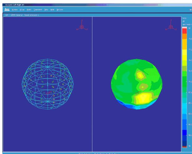
Fig. 9: Baroque violin: overall response (0 - 12500 Hz).
