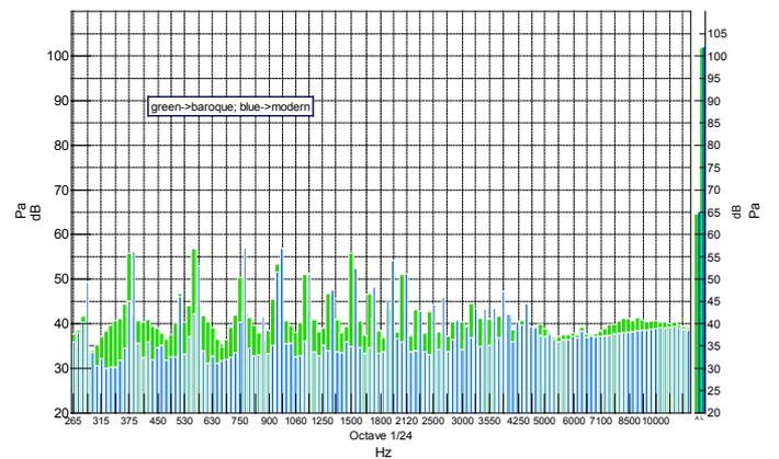
Fig. 4: Sound pressure vs. frequency (1/24 of octave).
