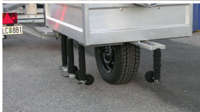
Fig 4. Free field mounted microphones on the test tyre unit of the trailer according to the CPX standard. The hood on the support trailer was not yet mounted at these measurements.
