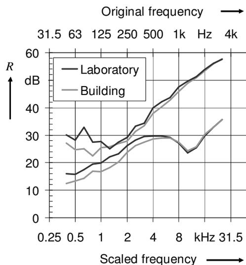
Fig. 9 Mean value of the sound reduction index of a heavy (upper two curves) and a lightweight element (lower two curves) in six different laboratory and building geometry simulations
