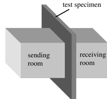
Fig. 7 Basic idea for the investigation of the influence of structure-borne modes on the specimen.
