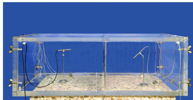
Fig. 4 Scale model of a wall test facility made of acrylic glass.
