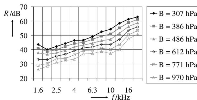
Fig. 3 Sound reduction index  $R$  of a double-shell specimen consisting of a 3 mm hard board ( $m'' = 2.55 \text{ kg/m}^2$ ) and a plastic film ( $m'' = 0.25 \text{ kg/m}^2$ ) with 34 mm spacing at different static pressures  $B$ .
