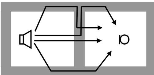
Fig. 1 Sound transmission between two adjacent rooms.
