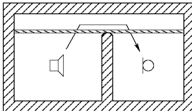
Fig. 11 Layout of a test facility with a flanking test object installed alongside the test facility wall (top view).
