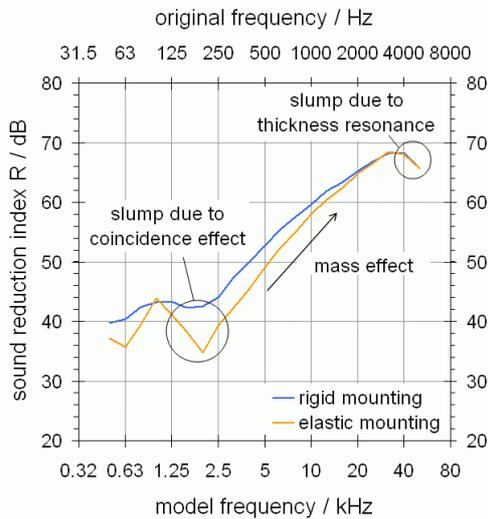
Fig. 5 Sound reduction index of a 24 cm lime brick wall.
