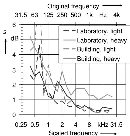
Fig. 10 Standard deviation of the sound reduction index of a heavy and a lightweight element in six different laboratory and building geometries.
