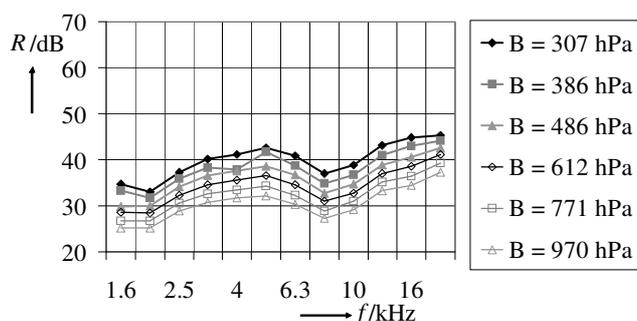
Fig. 2 Sound reduction index  $R$  of a 1.5 mm aluminium plate at different static pressures  $B$ .
