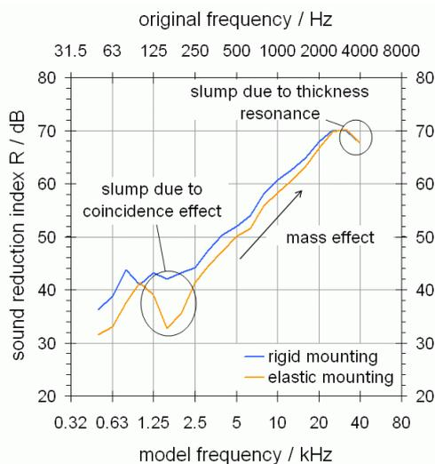
Fig. 6 Sound reduction index of a 25 mm acrylic glass wall.
