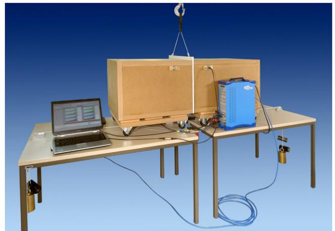
Fig. 8 Measurement setup for the investigation of the influence of structure-borne modes on the specimen.
