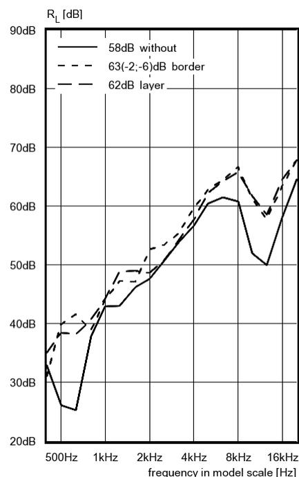
Fig. 12 Flanking sound reduction of a single-leaf test object with cavity damping varied (without damping, with strips in front of the cavity floor, ceiling and walls (border) and with one layer behind the test object); cavity depth 5 cm.
