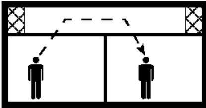
Fig. 13 Layout of a test facility with a suspended ceiling.
