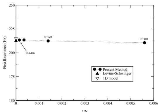
Figure 3: Convergence of the first impedance peak w.r.t. the number of boundary elements.
