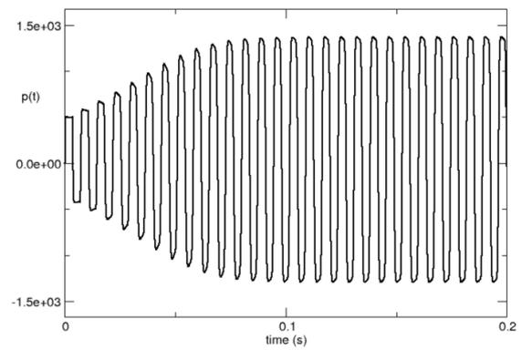
Figure 10: Pressure at the clarinet input section in playing condition. Lowest tone.
