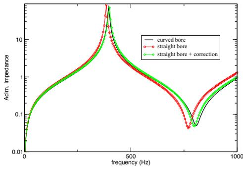
Figure 6: Effect of the curvature for the elbow of a tenor saxophone.
