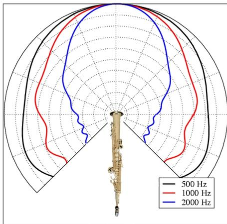
Figure 7: Directivity pattern of a soprano saxophone.
