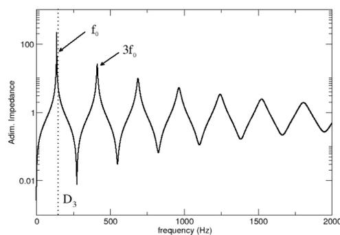
Figure 4: Dimensionless input impedance for a clarinet.
