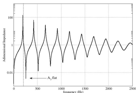
Figure 5: Dimensionless input impedance for a soprano saxophone.
