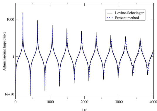
Figure 2: Dimensionless input impedance for a cylindrical tube ( $L = 1 m.$ ,  $r = 1 cm.$ ). Comparison with the Levine & Schwinger theory.
