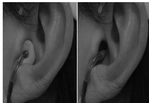
Figure 2: Example of the microphone positioning for the blocked-entrance measurements (left picture) and the open-entrance measurements (right picture).
