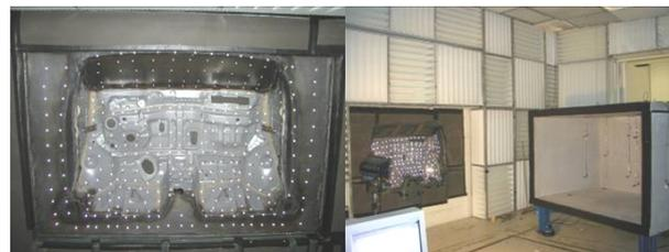
Figure 3: Bare dash panel experimental setup.
