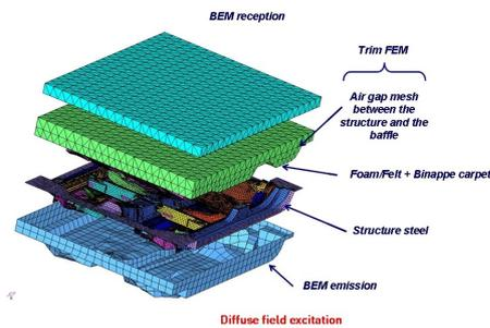
Figure 17: Floor trim FEM Transmission Loss model
