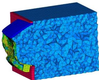
Figure 8: Complete Dash trim FEM model with cavity.
