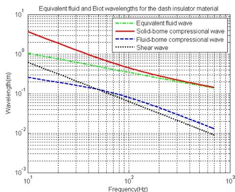
Figure 1: Biot wavelengths for the dash trim.
