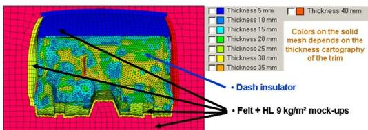
Figure 7: Dash trim FEM model with mock-ups.
