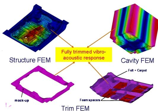
Figure 13: Complete floor trim FEM model with cavity
