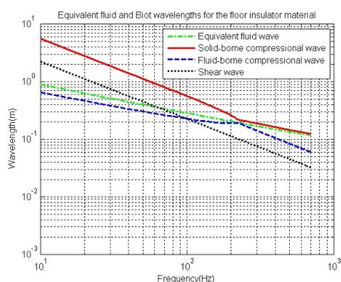
Figure 2: Biot wavelengths for the floor trim.
