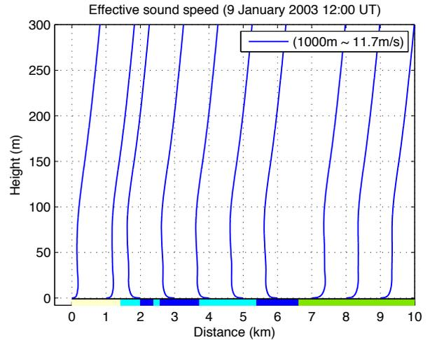
Figure 8. Effective speed of sound as a function of distance and height.
