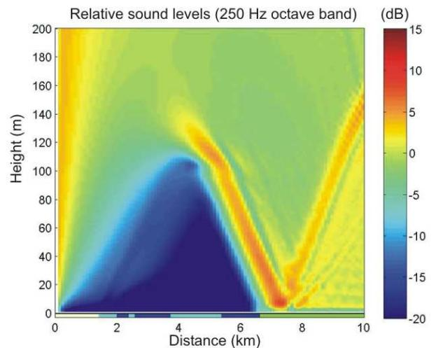
Figure 10. Results of the acoustical model, i.e. excess attenuation levels, for the 250 Hz octave band for the profiles as shown in Figure 8.
