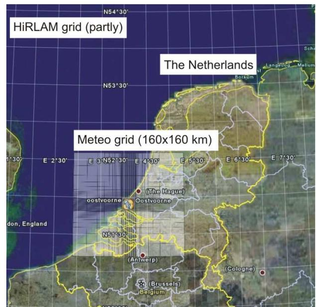
Figure 2. Overview of HiRLAM grid and meteorological model grid (centered around Oostvoorne).
