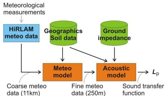
Figure 1. Structure of the meteorological-acoustical model.
