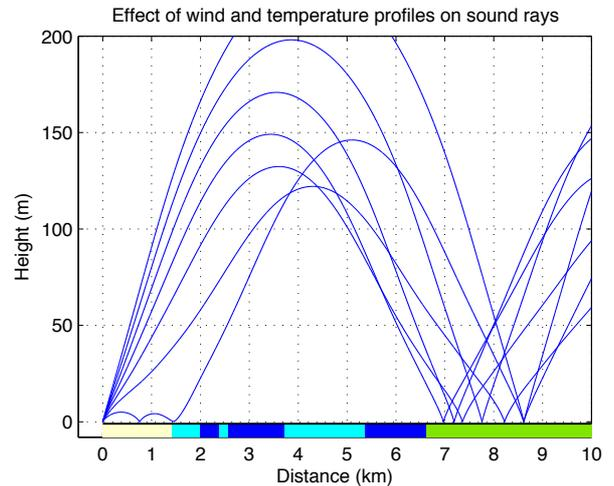
Figure 9. Curved sound rays due to the speed of sound profiles as shown in Figure 8.
