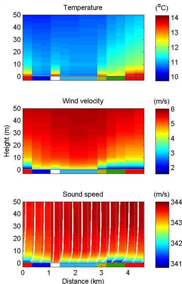
Figure 5. Example of temperature, wind velocity and resulting sound speed as a function of distance and height along the line for a sound propagation calculation.
