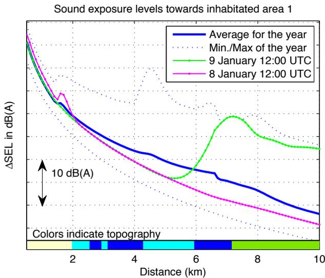
Figure 7. Averaged A-weighted sound pressure levels and levels for the meteorological situation at Januari 9<sup>th</sup> and 8<sup>th</sup> in the direction of inhabited area 1.
