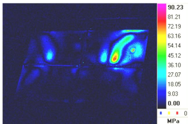
Fig.6 Results of non-contact stress distribution measurement with lock-in thermography. Excitation frequency 85,06 Hz
