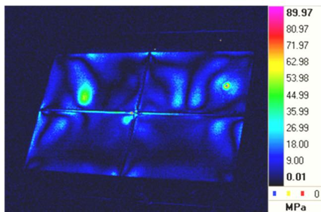
Fig.5 Results of non-contact stress distribution measurement with lock-in thermography. Excitation frequency 52,54 Hz
