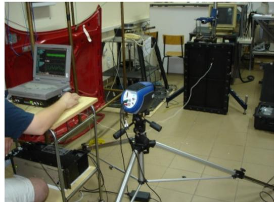
Fig.3 Measurement system with infrared thermographic camera for lock-in-thermography
