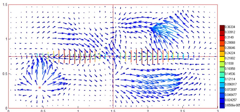
Fig.1 Distribution of structural intensity vectors for simply supported ribbed rectangular plate. Excitation frequency 52 Hz.
