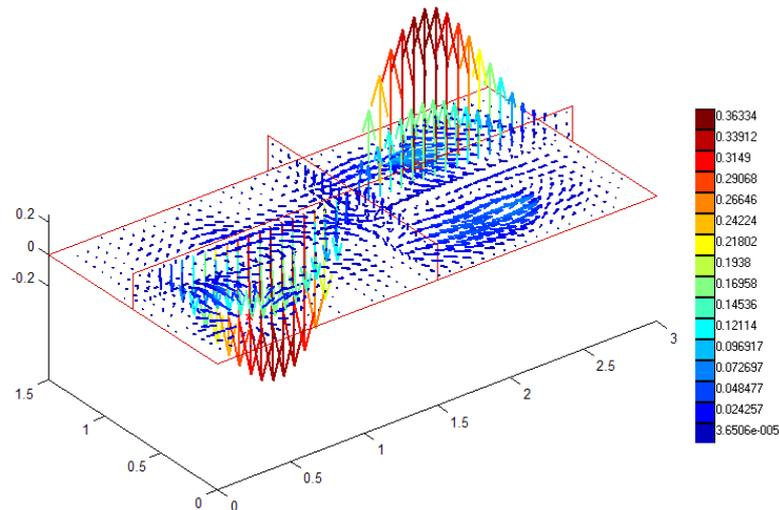
Fig.2 Distribution of structural intensity vectors for simply supported ribbed rectangular plate. Excitation frequency 52 Hz.
