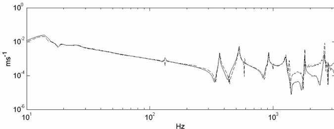
Fig. 10 Coupled velocity: Directly measured (solid line) and predicted from blocked force and coupled mobility (dashed line)
