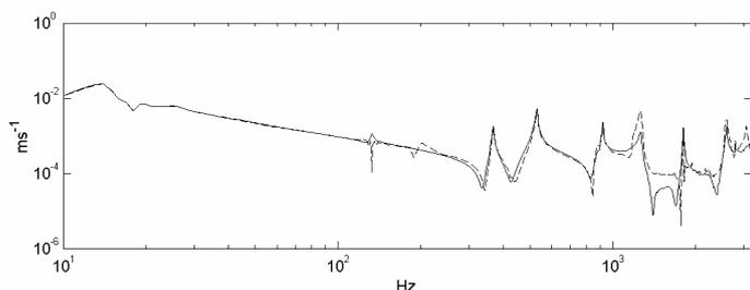
Fig. 6 Coupled velocity: Directly measured (solid line) and predicted from blocked force and coupled mobility (dashed line)
