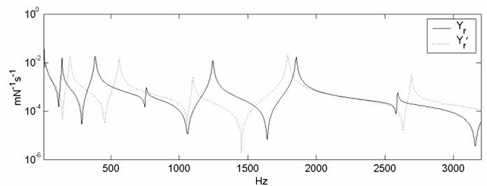
Fig. 5 Receiver mobilities: Receiver mobility (solid line) and reference beam mobility (dotted line)
