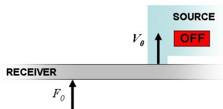
Fig. 9 Coupled transfer mobility measurement.
