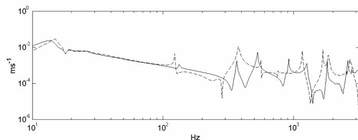
Fig. 2 Coupled velocity: Directly measured (solid line) and predicted from source and receiver mobilities and free velocity “conventional method” (dashed line)
