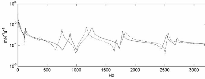
Fig. 4 Measured (solid line) and predicted (dotted line) coupled mobility for two beams connected by two bolted square contacts. One of two contact points shown.
