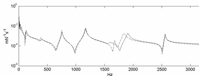
Fig. 3 Measured (solid line) and predicted (dotted line) coupled mobility for two beams connected by two sliding square contacts. One of two contact points shown.
