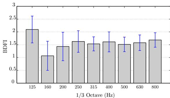
Figure 1: Calculated mean BDFI value and standard deviations - Room dimensions:  $l_x=11.5\text{m}$ ,  $l_y=8.69\text{m}$ ,  $l_z=4.03\text{m}$  - 247 patches over a surface of  $0.96\text{m} \times 1.5\text{m}$  centered on  $x=6\text{m}$   $y=0\text{m}$   $z=1.75\text{m}$  - Patch dimensions :  $\Delta X = 0.08\text{m}$ ,  $\Delta Z = 0.074\text{m}$  - Source position  $x=2\text{m}$ ,  $y=4\text{m}$ ,  $z=1\text{m}$  - Cut-off frequency: 187Hz
