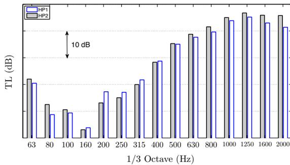
Figure 8: Measured Transmission Loss of a plasterboard panel with two source positions
