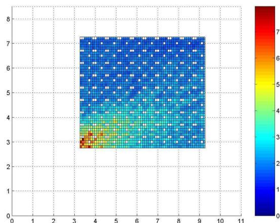
Figure 3: xy spatial BDFI distribution at 2000Hz - Room dimension :  $L_x=11.5\text{m}$   $L_y=8.69\text{m}$   $L_z=4.03\text{m}$  - Cutoff frequency: 187 Hz - Source Location :  $x=2\text{m}$   $y=2\text{m}$   $z=0.5\text{m}$
