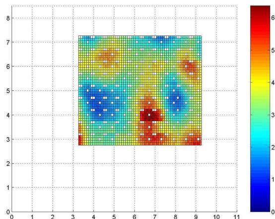
Figure 2: xy spatial BDFI distribution at 80Hz - Room dimension :  $L_x=11.5\text{m}$   $L_y=8.69\text{m}$   $L_z=4.03\text{m}$  - Cutoff frequency: 187 Hz - Source Location :  $x=2\text{m}$   $y=2\text{m}$   $z=0.5\text{m}$
