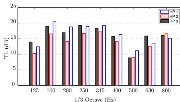
Figure 6: TL of a double aluminum panel (2mm and 1.5mm thickness, separated by 3cm of air) for three source positions
