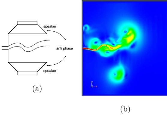
Figure 1: (a) Schematic illustration of a jet deflection experiment. (b) An oscillating jet numerically simulated.
