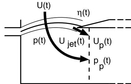
Figure 3: Flows and pressure near the pipe mouth.
