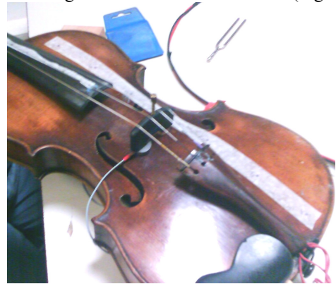
Fig. 11: Micro load cell under the bridge.
