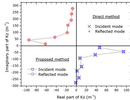
Fig. 3 Axial wavenumbers of dissipative muffler with perforated duct for an excitation frequency of 3.2 kHz.
