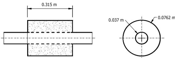
Fig. 2 Geometry of dissipative muffler.
