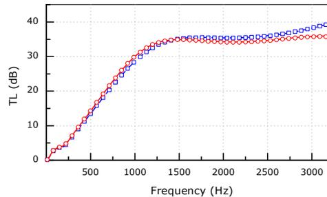
Fig. 6 TL of dissipative muffler: —, direct method with perforations; ○○○, proposed method with perforations; ---, direct method without perforations; □□□, proposed method without perforations.
