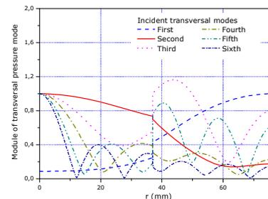
Fig. 5 Modulus of first transversal modes at a frequency of 3.2 kHz in Configuration 1.
