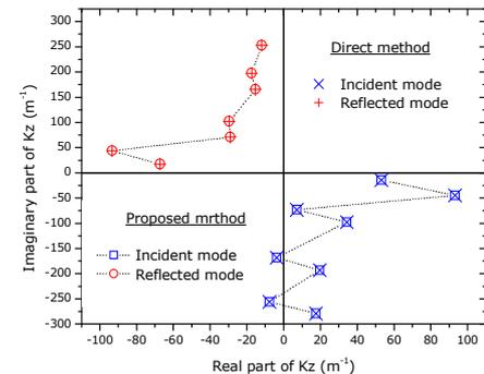
Fig. 4 Axial wavenumbers of dissipative muffler without perforated duct for an excitation frequency of 3.2 kHz.
