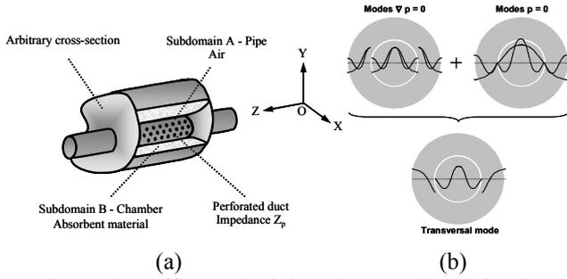
Fig. 1 (a) Muffler and subdomains considered for the application of the component mode synthesis approach. (b) Substructuring scheme used to calculate transversal modes.
